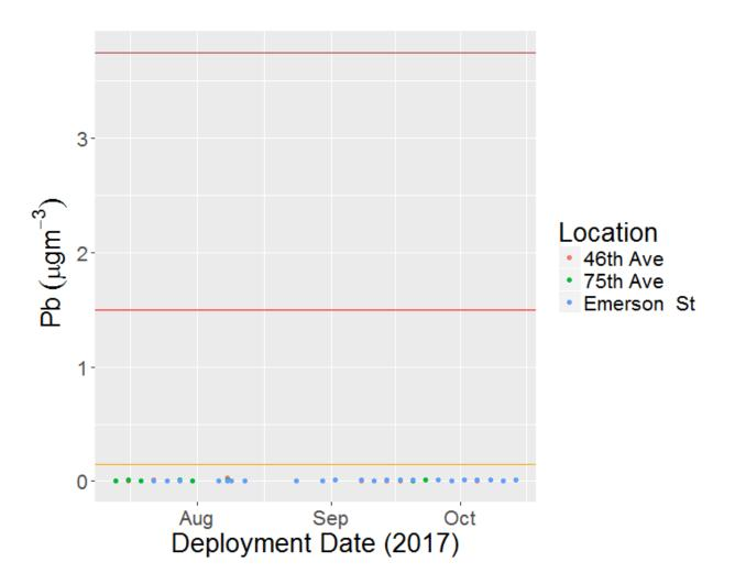
The orange horizontal line represents the Ambient Benchmark Concentration of **lead** (ABC = 0.15 ugm<sup>-3</sup>). The red and brown horizontal lines represent 10x ABC = 1.5 ugm-3 and 50x ABC = 7.5 ugm-3 respectively. **1.4% of the analyzed samples were below the detection limit (LOD = 0.003 ugm-3).**
