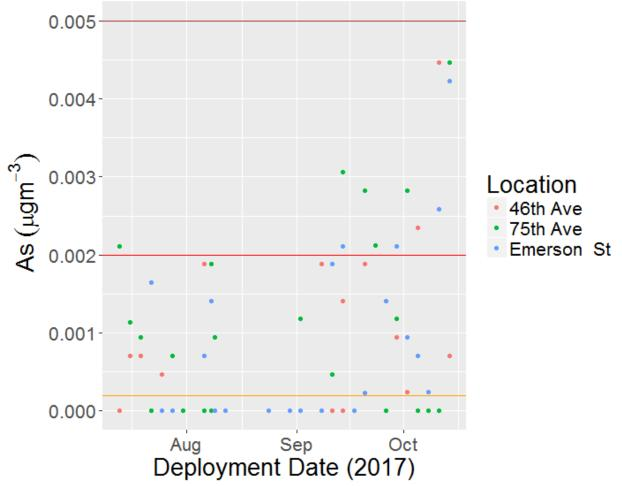
The orange horizontal line represents the current Ambient Benchmark Concentration of **arsenic** (ABC =  $0.0002 \text{ ugm}^{-3}$ ). The red and brown horizontal lines are  $10x \text{ ABC} = 0.002 \text{ ugm}^{-3}$  and  $50x \text{ ABC} = 0.01 \text{ ugm}^{-3}$  respectively. **65.7% of the analyzed samples were below the detection limit (LOD = 0.001 \text{ ugm}^{-3}).**
