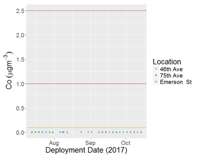
The orange horizontal line represents the Ambient Benchmark Concentration of **cobalt** (ABC = 0.1 ugm<sup>-3</sup>). The red and brown horizontal lines represent 10x ABC = 1.0 ugm-3 and 50x ABC = 5.0 ugm-3 respectively. **12.9% of the analyzed samples were below the detection limit (LOD = 0.0008 ugm-3).**
