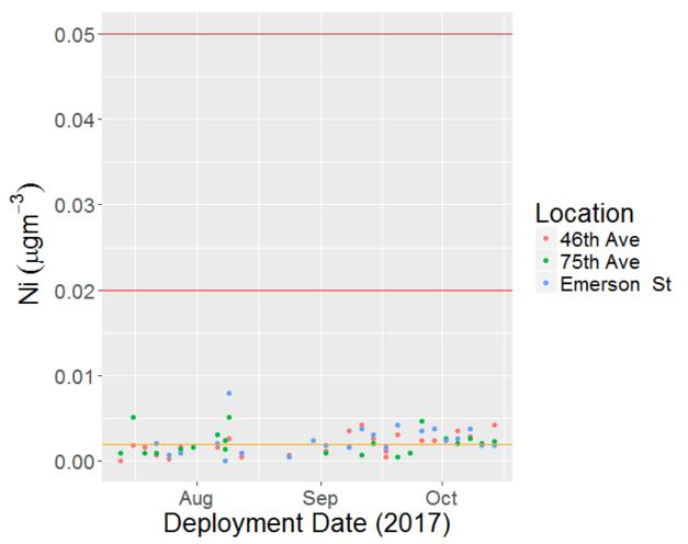
The orange horizontal line represents the Ambient Benchmark Concentration of **nickel** (ABC =  $0.002 \text{ ugm}^{-3}$ ). The red and brown horizontal lines represent 10x ABC =  $0.02 \text{ ugm}^{-3}$  and 50x ABC =  $0.1 \text{ ugm}^{-3}$  respectively. **25.7% of the analyzed samples were below the detection limit (LOD = 0.001 \text{ ugm}^{-3}).**
