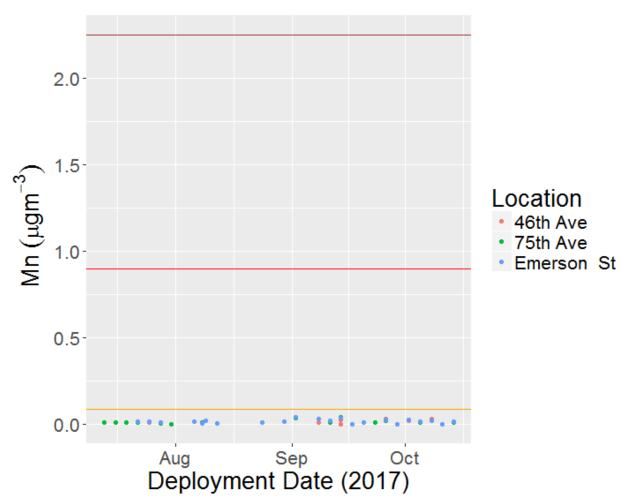
The orange horizontal line represents the Ambient Benchmark Concentration of **manganese** (ABC = 0.09 ugm<sup>-3</sup>). The red and brown horizontal lines represent 10x ABC = 0.9 ugm-3 and 50x ABC = 4.5 ugm-3 respectively. **0% of the analyzed samples were below the detection limit (LOD = 0.0003 ugm-3).**
