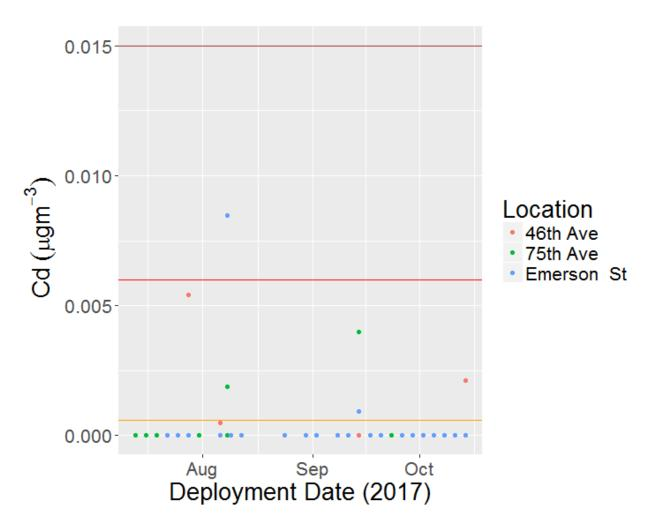
The orange horizontal line represents the Ambient Benchmark Concentration of **cadmium** (ABC =  $0.0006 \text{ ugm}^{-3}$ ). The red and brown horizontal lines represent  $10x \text{ ABC} = 0.006 \text{ ugm}^{-3}$  and  $50x \text{ ABC} = 0.03 \text{ ugm}^{-3}$  respectively. **91.4% of the analyzed samples were below the detection limit** (LOD = 0.0006 ugm-3).
